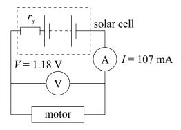
(a) Show that, in this circuit, the internal resistance of the solar cell is  $64.3~\Omega$ .
