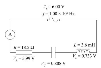
(b) Explain why the numerical values of  $V_R$ ,  $V_C$  and  $V_L$  in the diagram do not add up to the numerical value of the supply voltage.
