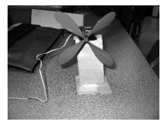
Jill is making a model wind turbine. It includes a generator constructed from a strong horseshoe magnet and a coil of wire, with 500 turns.
